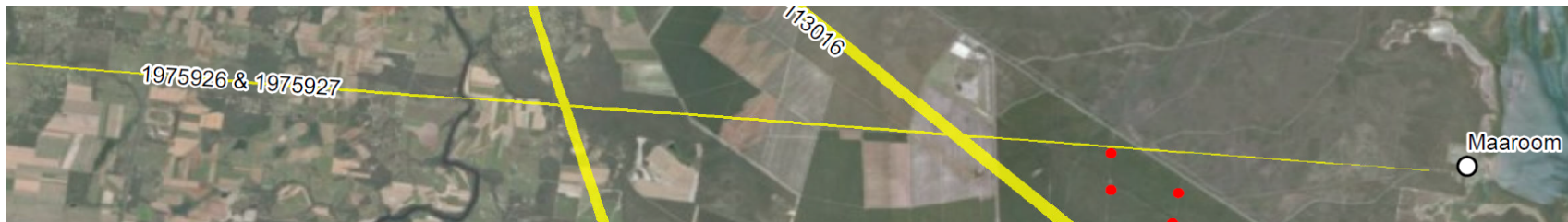
Figure 6 NBN Microwave Link Maaroom to Mungar Second Fresnel Zone 10 m from Turbine
