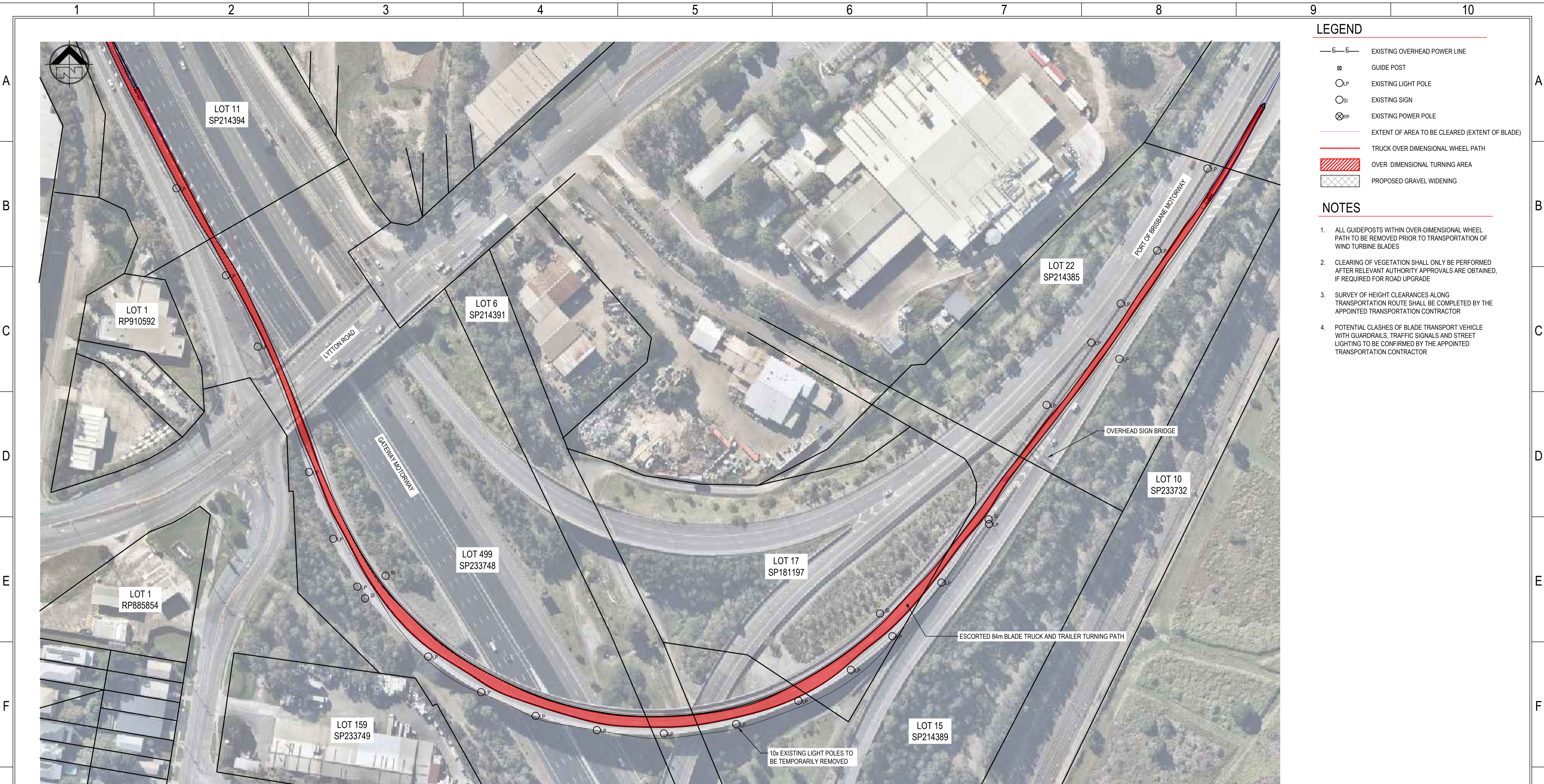
INTERSECTION 3 - PORT DRIVE / GATEWAY MOTORWAY, MURARRIE INTERSECTION PLAN - 84m BLADE TRUCK AND TRAILER
